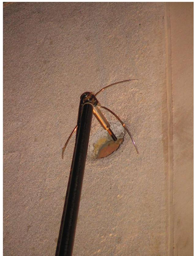
Figure 5. View of the top part of the carbon fibre pole fitted with tripod and microphone – the microphone points to the opening of a pot.
